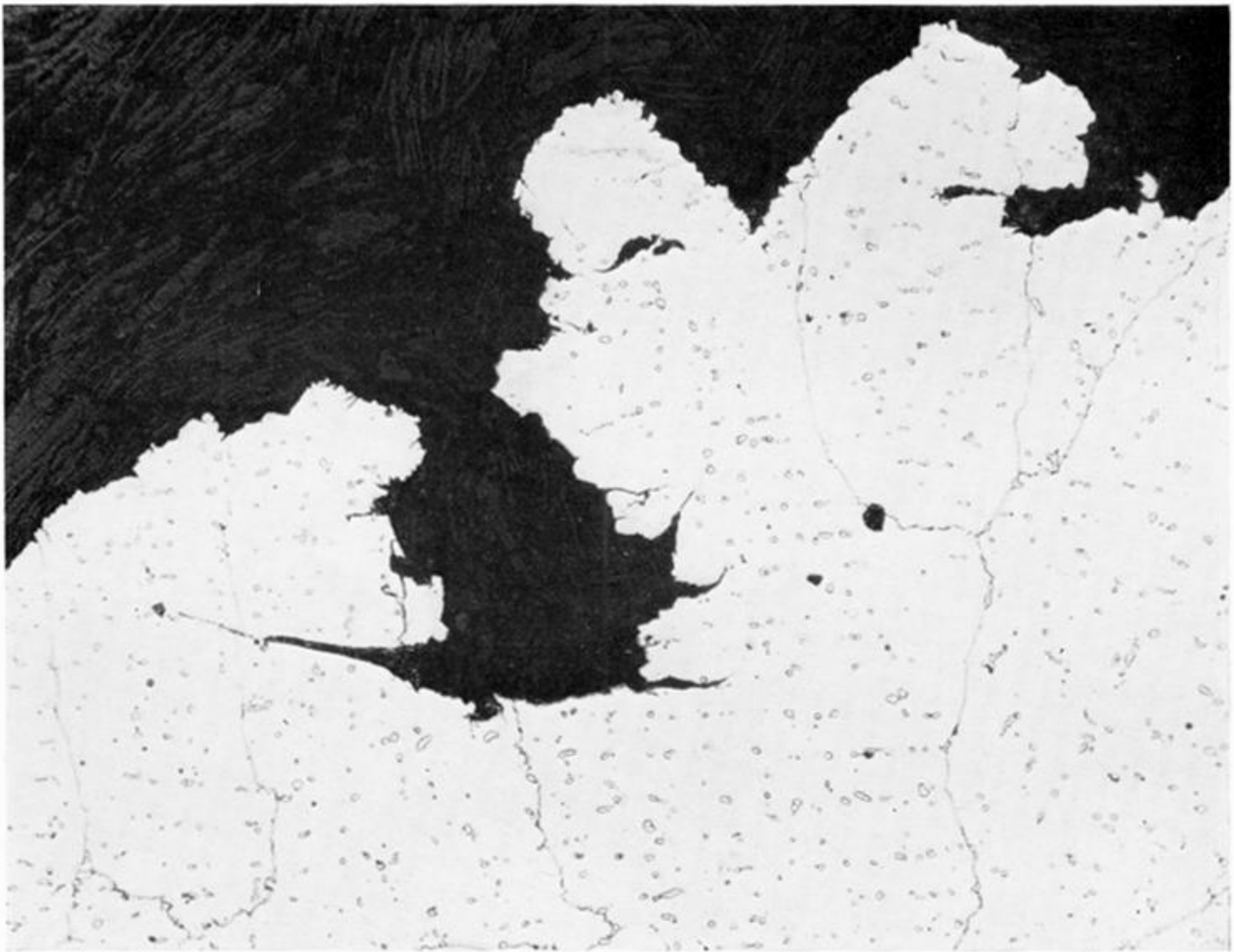
FIGURE 9. Form of cracking in peak remaining between erosion pits (cast no. 7 alloy). (Magn. \times 110 .)
